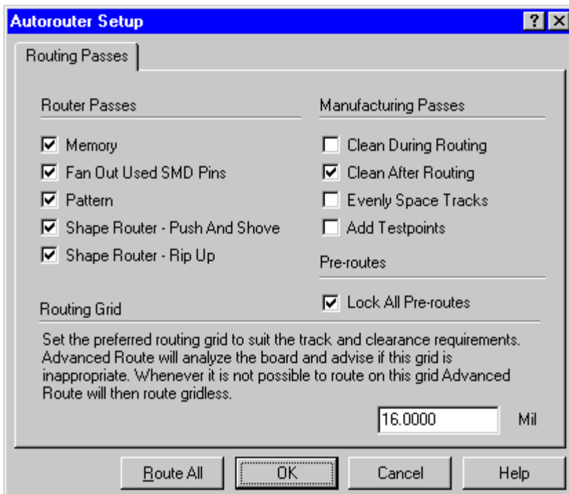
Figure 21 Autorouter Setup dialog box
