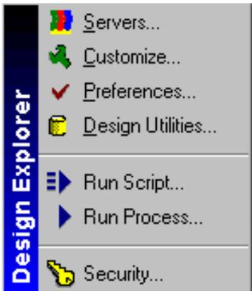
The **System** Menu provides commands for configuring the Design Explorer. You can access these commands by clicking on the down pointing arrow
