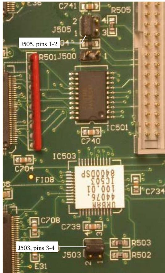
Figure 4: Jumper Positions, Component Locations: Standard DSP board
